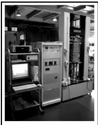
Figure 2. High-temperature tension/compression test machine
